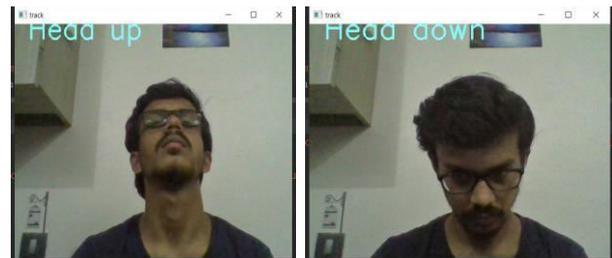
Takes 3D coordinates of facial landmarks and estimates the rotational and translational vectors at the nose tip head\_pose\_estimation.py is used for finding where the head is facing.
