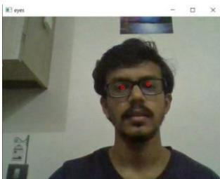
Takes 3D coordinates of facial landmarks and estimates creates a new black mask using NumPy of the same dimensions as our webcam frame. Store the (x, y) coordinates of the points of the left and right eyes from the keypoint array shape and draw them on the mask. it creates an image with the area between those points filled with that color. and later we can track the colored eyes in the eyeball tracking .eye\_tracker.py is used to track eyes. However, it was written using dlib.
