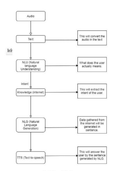
Fig-3: Internal Working
