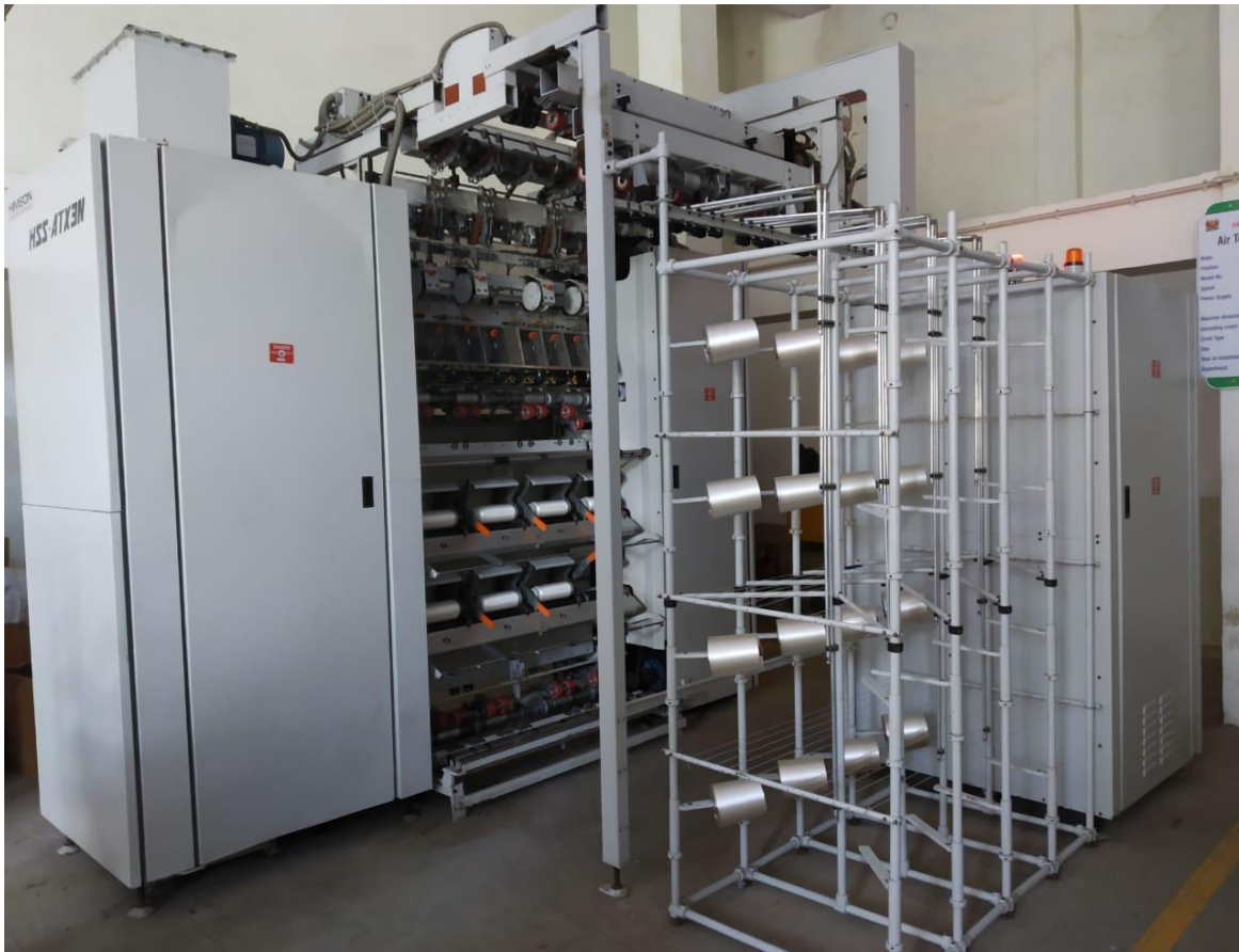
Air texturing Machine Parameters suitable for viscose filament yarn.
