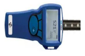
Fig. 7 Air Quality Indicator It is a device to determine the quality of air. It represent the amount of Carbon, Nitrogen and Sulphur present in the air before and after the filteration chambers.
