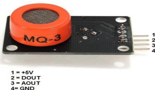
Figure 1 MQ-3 sensor for alcohol detection
