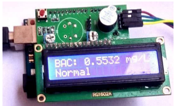
Figure 6.LCD Output of alcohol detection when driver is not in drunken state
