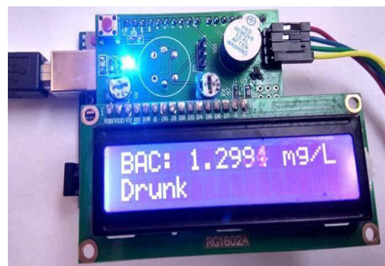
Figure 7 LCD Output of alcohol detection when driver in drunken state
