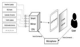
Fig 7: Proposed Block Architecture of Smart Mirror
