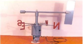
Fig. 3: Potentiometric wind vane
