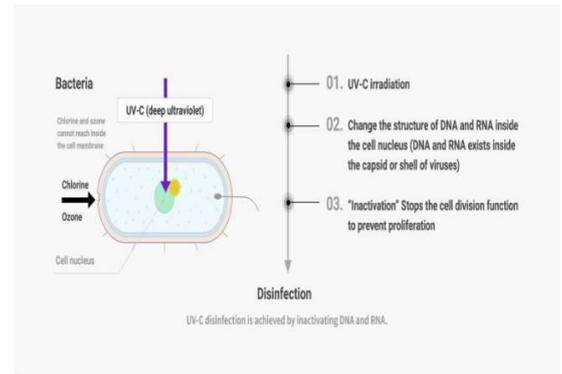
Fig 2: Working of UV-C light
