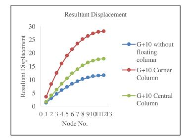
Figure 5: Resultant displacement for G+10 Building
