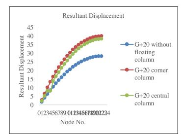
Figure 6: Resultant displacement for G+20 Building
