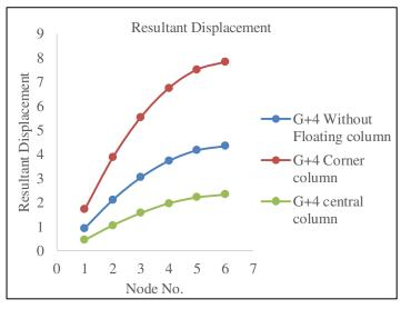
**Figure 4:** Resultant displacement for G+4 Building
