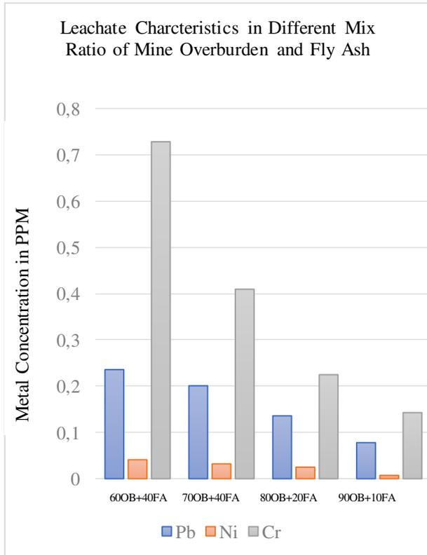
**Fig-4:** Leachate Characteristics in different mix ratio of mine overburden and fly ash
