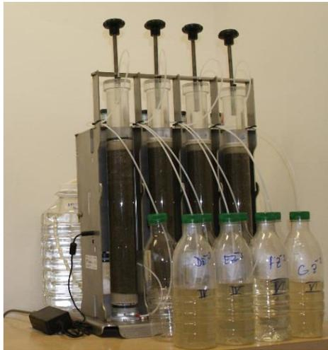
Fig-2: Laboratory setup for column test
