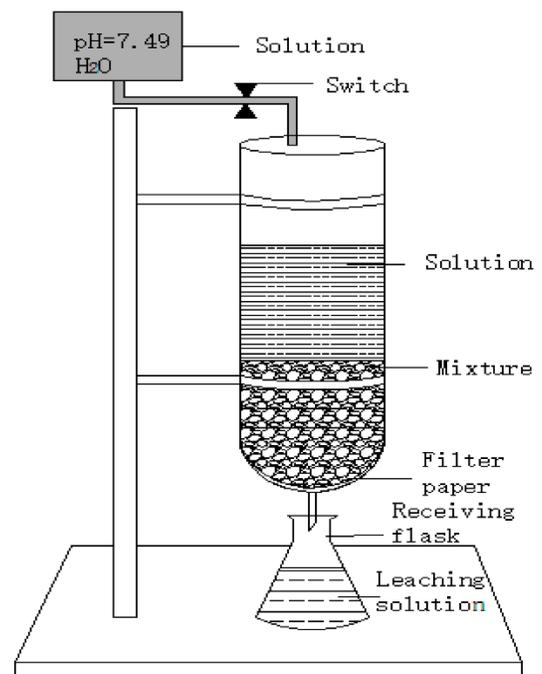
Fig.-1: Typical arrangement of column test
