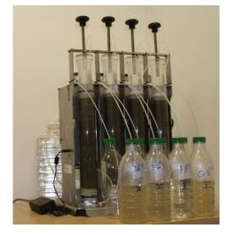
Fig-2: Laboratory setup for column test
