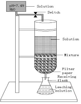
Fig.-1: Typical arrangement of column test
