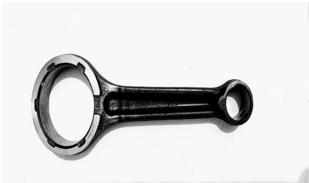
Fig. 3.3 Actual photograph of Hero Splendor plus Connecting Rod.
