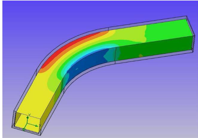
**Fig 6.1 C in curve duct FD analysis of air flow**
