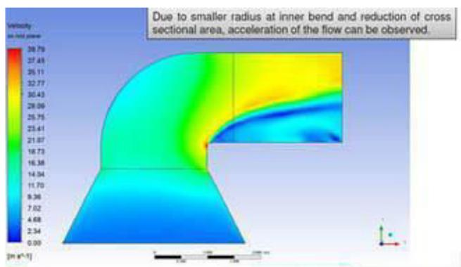
**Figure 6.3** cfd analysis of air in the diffuser
