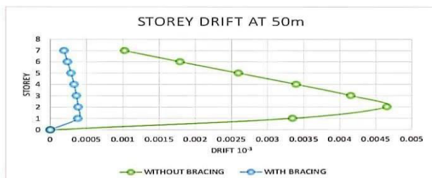
Graph :14 Variation of storey drift with bracing and without bracing for 100kg rdx at 50m stand-off distance.
