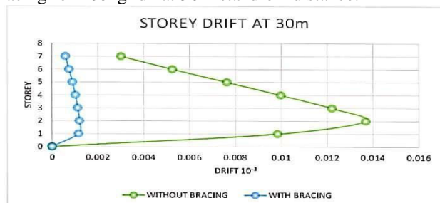
Graph:10 Variation of storey drift with bracing and without bracing for 100kg rdx at 30m stand-off distance.
