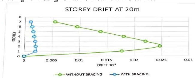
Graph:8 Variation of storey drift with bracing and without bracing for 100kg rdx at 20m stand-off distance.
