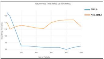
Fig. 5 Round Trip Time MPLS vs Non-MPLS Topology 2
