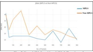
Fig. 7 Jitter MPLS vs Non-MPLS Topology 2
