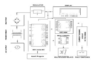
Fig.1 Block diagram of the model
