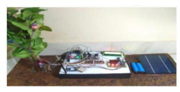
In this system we haveused multiple sensors like pH sensor, fire sensor, accelerometer, ultrasonic sensor.
