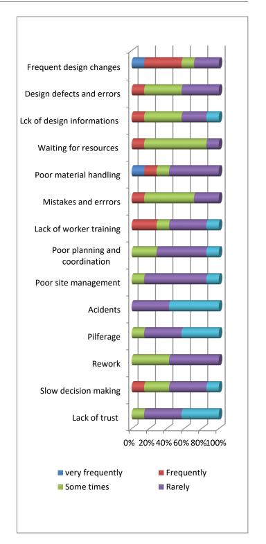
Fig -5 Occurrences of waste in the construction industry
