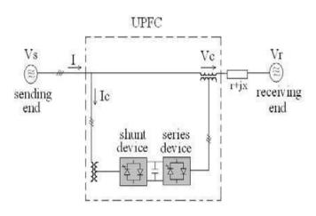
Fig. 2 Basic Operation of UPFC
