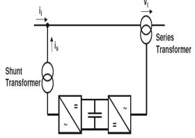
Fig. 1 Principle configuration of an UPFC
