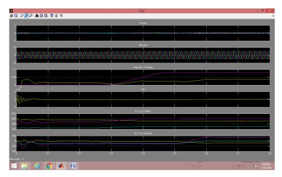
Fig.4.2 Series voltage injection in SSSC mode
