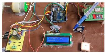
Case 2: when a alcohol consumed person enter in and the level is detected by sensor and level is goes beyond 30 percentage cars Engine will be automatically OFF. Refer fig.5
