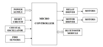
Fig-1: Architecture of Microcontroller
