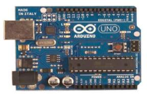
Fig-2: Arduino UNO Microcontroller
