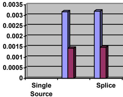
Fig 1.8. Bar chart Output amplified Signal Power and ASE noise in single pumping analysed with single source of 1550nm
