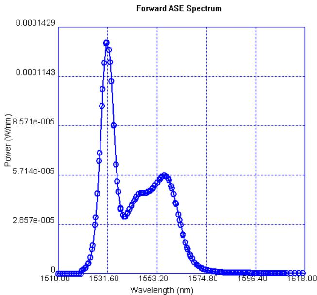
Fig. 1. 6. Forward ASE Noise Characteristics (after filter) of two EDFAs are connected by connector
