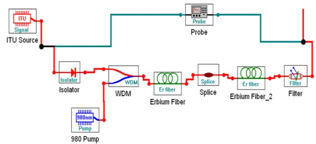
Fig 1.3. Simulated model of two EDFAs are connected with splice technique using single Pumping scheme
