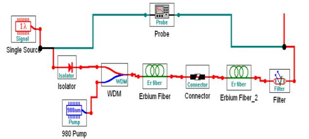
Fig 1.4. Simulated model of two EDFAs are connected with connector using single Pumping scheme
