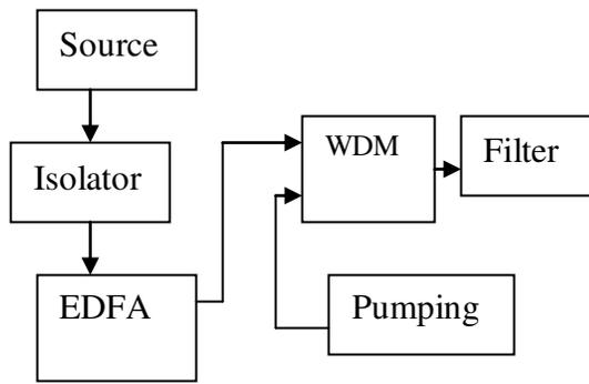
Fig 1.2 .Block Diagram of single stage (forward) pumping
