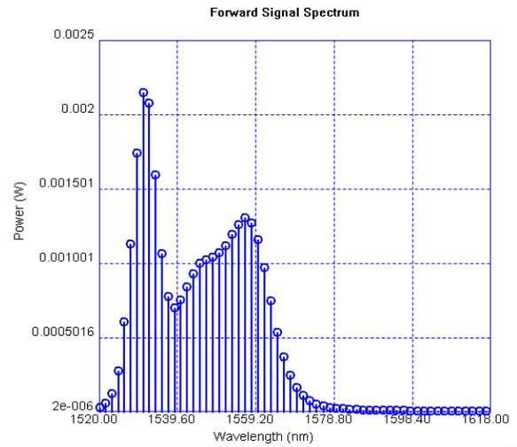
Fig 1.7. Forward Signal power characteristics in two EDFAs connected by connector
