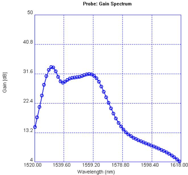
Fig.1.5 Gain characteristics of single pumping two EDFAs are connected by connector of length 10m and pump power 0.12w.
