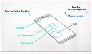
Fig 1: Working of location based AR system in a smartphone
