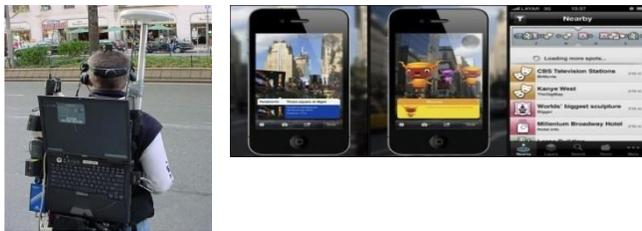
Figure 2: Mobile AR: (a) user with Mobile AR system backpack; (b) example of AR application that uses mobile devices.
