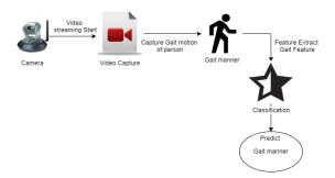
Fig1. Proposed System Architectural diagram
