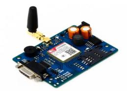
Fig -5: GSM Module
