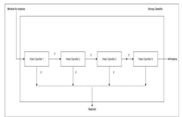
Fig 1: Concept of Cascade Classifier
