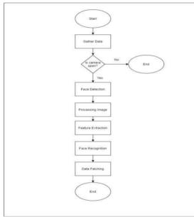
Fig 2: Flow chart of face recognition system
