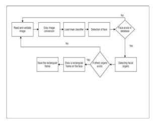
Fig 3: Flow chart of Face Detection Process
