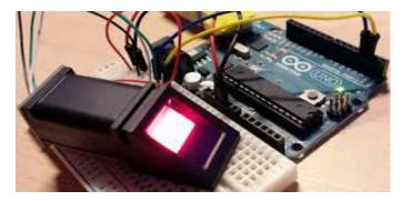
Figure 6 Module for CustomerEnrollment into theFingerprint System (Source:<u>https://www.electroschematics.com/h</u> <u>ow-to-use-fingerprint-identification-modules/</u>)
