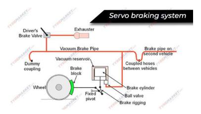
Fig 4.1 Servo braking system
