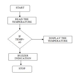
Fig 5: Temperature Monitoring
