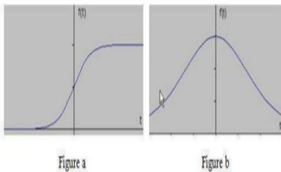
**Fig: trend of signal and its derivative**
