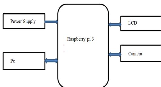
Hardware interfacing module consists of hardware components such as Raspberry Pi 3 ,personal computer to process open CV code to Raspberry Pi3, Power supply, HDMA2 vga cabel,
