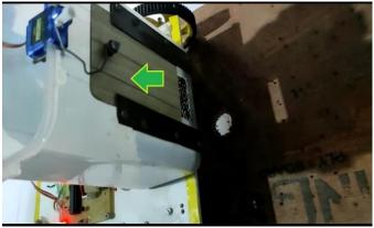
The output shaft of the servomotor is capable of traveling somewhere around 180 degree. A 1.5ms pulse is provided to servomotor which makes the motor turn 90-degree position, which lifts the slat and thus allows material to fall on detected pothole.
