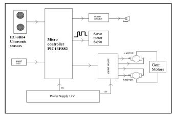
Fig: Block Diagram of Pothole Filling System
