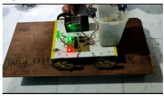
The path hole will be detected with the help of ultrasonic sensor. The sensors will continuously transmit an ultrasonic wave form the transmitter and then wave will travel in air and reflect back to the sensor's receiver. If there is any disturbance or differences between transmitted and received wave (i.e. if pulse width is more than 25ms), the microcontroller will detect the Pothole and the machine will stop.
