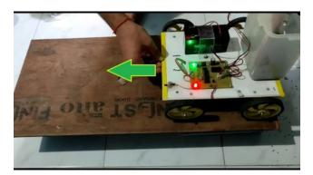
When the machine is in auto mode, the machine will automatically move forward with the help of gear motor. It will move forward until it detects the path holeusing ultrasonic sensor.
