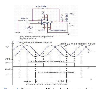
Figure 4: Comparator and its input, output wave shape
