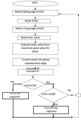
Figure 6: Flow chart of the microcontroller program
