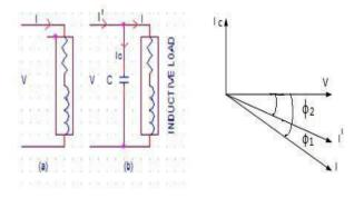
Figure 1 : Power factor improvement circuit and phasor diagram
