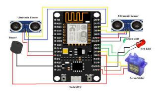
Fig -1: Hardware Arrangement and Physical Connection
