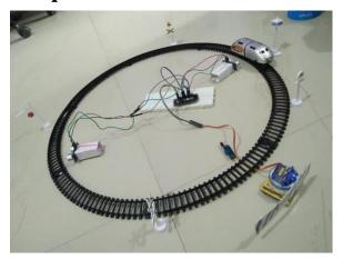
Fig -5: Train is Arrived from Sensor-1 and Gate is Close
