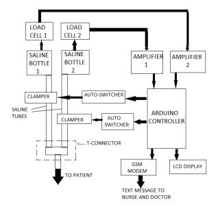
Fig 4: System architecture
