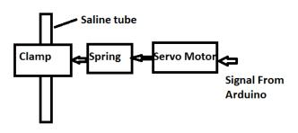
Fig 3: auto switching mechanism
