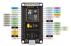
Fig 2.2: pin description of Nodemcu.
