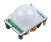
Fig 3.5: PIR sensor module
