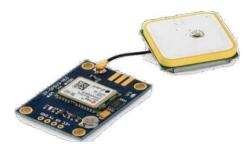
Figure 5: Global Positioning System Module
