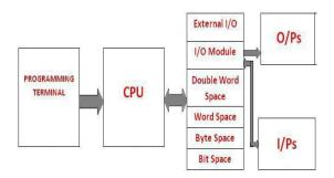
Fig.1. Basic Block Diagram of PLC
