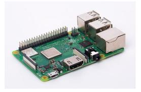
Fig 1: Raspberry Pi-3B plus model
