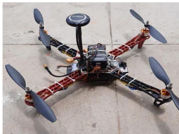
Fig.4 Quadcopter using PX4 board
