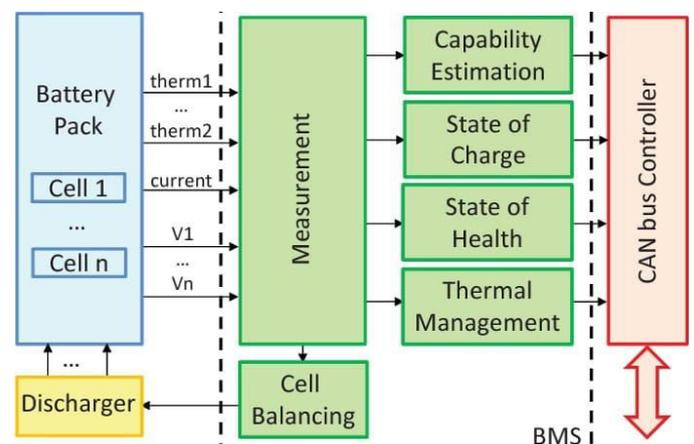
This is the diagram of battery management system (BMS), Primary functions of the BMS:
