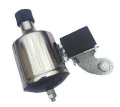
This is used to generate a 12v dc while driving a cycle. In our project we used two generators connected in series to generate 24vdc to charge 24v batteries. Maximum output of a genertor is of 24 watts at 300 rpm, which is used to charge the batteries.at 1.2Amp current.
