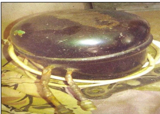
Fig. 4 Hermetically sealed compressor
