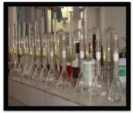
Fig -1: Arsenic concentration testing
