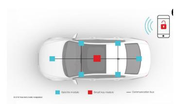
Fig. 1:A passive-entry passive-start architecture in a car. The number of satellite modules will vary, depending on system-level requirements
