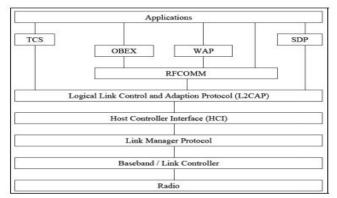
Figure 1.1 The Bluetooth Protocol Stack
