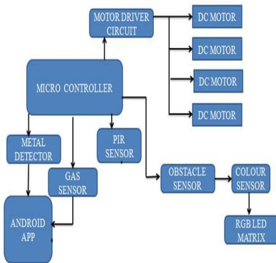
Figure:Architectural diagram of Camouflage Army Robot
