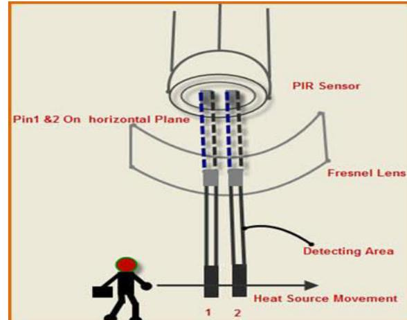
The PIR sensor internally is split into two halves, one half is positive and the other is considered as negative. Thus, one half generates one signal by detecting the motion of a hot body and other half generates another signal. The difference between these two signals is generated as output signal. Primarily, this sensor consists of Fresnel lens which are bifurcated to detect the infrared radiation produced by the motion of hot body over a wide range or specific area.
