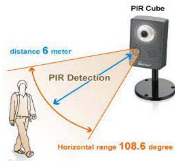
Whenever, human being (even a warm body or object with some temperature) passes through the field of view of PIR sensor, then it detects the infrared radiation emitted by a hot body motion. Thus, the infrared radiation detected by the sensor generates an electrical signal that can be used to activate an alert system or buzzer or alarm sound.
