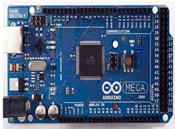
Figure: Arduino Mega Board
