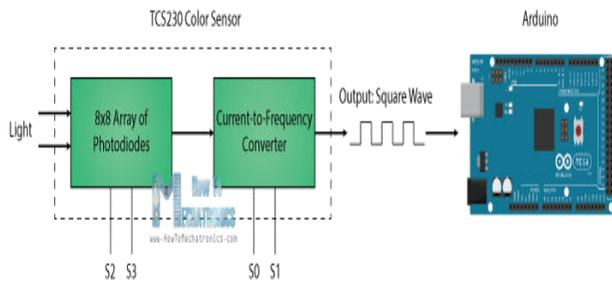
If we take a closer look at the sensor we can see how it detects various colors. The photodiodes have three different color filters. Sixteen of them have red filters, another 16 have green filters, another 16 have blue filters and the other 16 photodiodes are clear with no filters.
