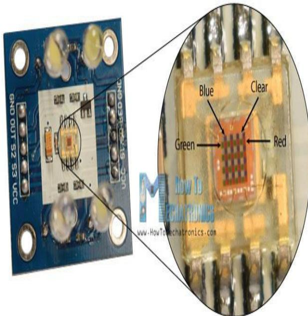
Each 16 photodiodes are connected in parallel, so using the two control pins S2 and S3 we can select which of them will be read. So for example, if we want to detect red color, we can just use the 16 red filtered photodiodes by setting the two pins to low logic level according to the table.
