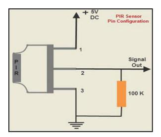
The pin configuration of the PIR sensor is shown in the figure.
