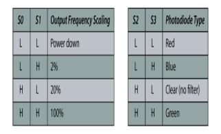
The sensor has two more control pins, S0 and S1 which are used for scaling the output frequency. The frequency can be scaled to three different preset values of 100 %, 20 % or 2%. This frequency-scaling function allows the output of the sensor to be optimized for various frequency counters or microcontrollers.
