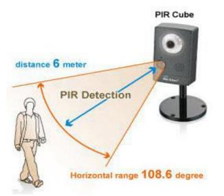
Whenever, human being (even a warm body or object with some temperature) passes through the field of view of PIR sensor, then it detects the infrared radiation emitted by a hot body motion. Thus, the infrared radiation detected by the sensor generates an electrical signal that can be used to activate an alert system or buzzer or alarm sound.
