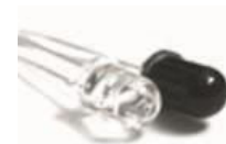
Fig. 3: IR diodes (Sender and Receiver sensor)
