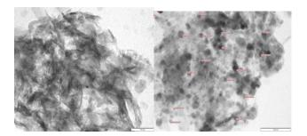
Figure 3. TEM micrographs of MgO and (Zn/Mg)O
