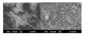
Figure 2.SEM micrographs of MgO and (Zn/Mg)O
